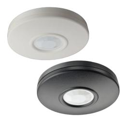
The ceiling mount, low profile panoramic DS936 PIR Detector uses alternate polarity pulse count. It also uses a pointable Fresnel lens to provide up to 7.5 m (24 ft) of coverage and can be mounted on the surface, or semi-flush directly to a ceiling or a standard octagonal electrical box.
